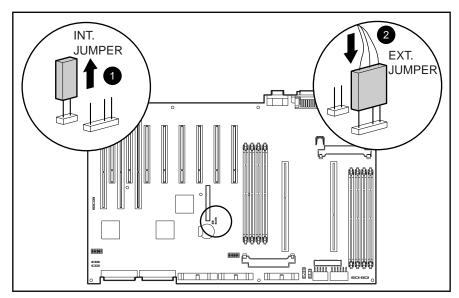
Figure 4-8. Battery jumper location and default settings
